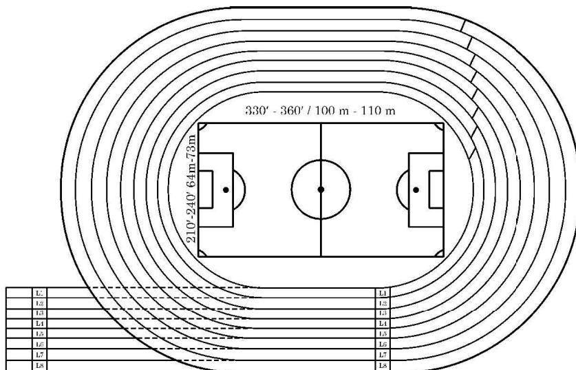
The length of innermost lane of the track is 400 m and each subsequent lane is 7.6 m longer than the preceding lane.
